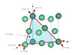
In the figure above a fcc unit cell with a (111) plane is shown. It gets obvious that the (111) plane has a threefold symmetry/ a triangular shape.
